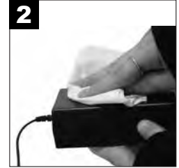
2 Wipe AC to DC adapter housing and cords with a dry cloth.
